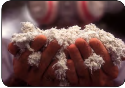
Asbestos fibres. Photo c/- Australasian Mine Safety Journal
