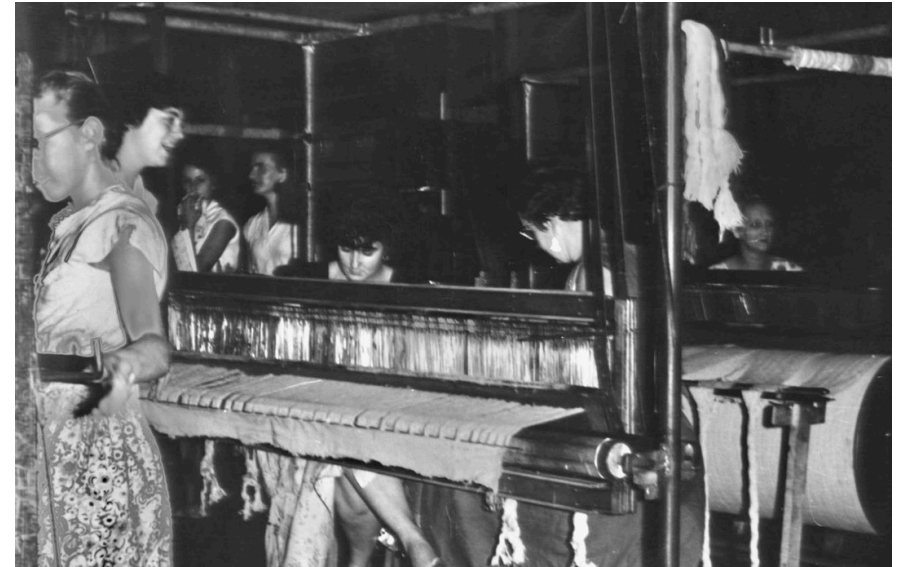
Figure 4. Women tying in the warp threads to the loom. This occurred at the start of each job on the loom. Depending on the fineness of the yarn (thread count) 1000 to 4000 thread would be individually tied in with reefknots. This was a skilled occupation.
